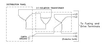
*Figure 8: Three Phase WYE (ungrounded) Distribution to a Three-Phase Delta/WYE Isolation Transformer*
